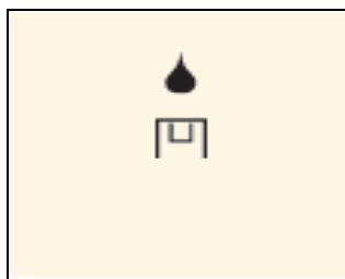
Figure 6.7 “Apply Sample” symbols on glucometer display
