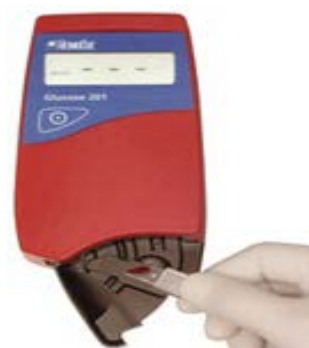
Figure 5.5 Placing the microcuvette in photometer
